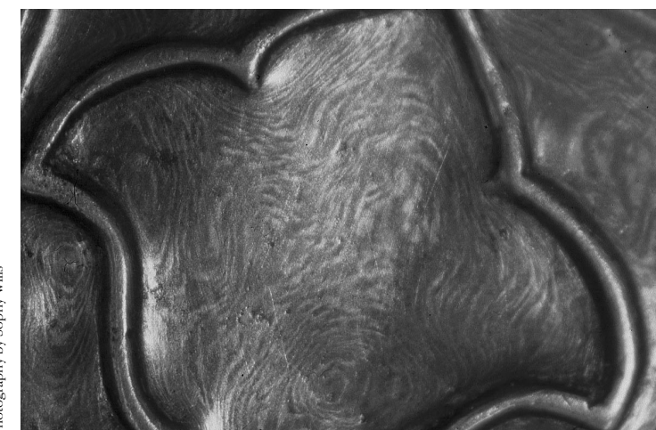
2.b Detail of the axehead after etching, showing watering pattern.
