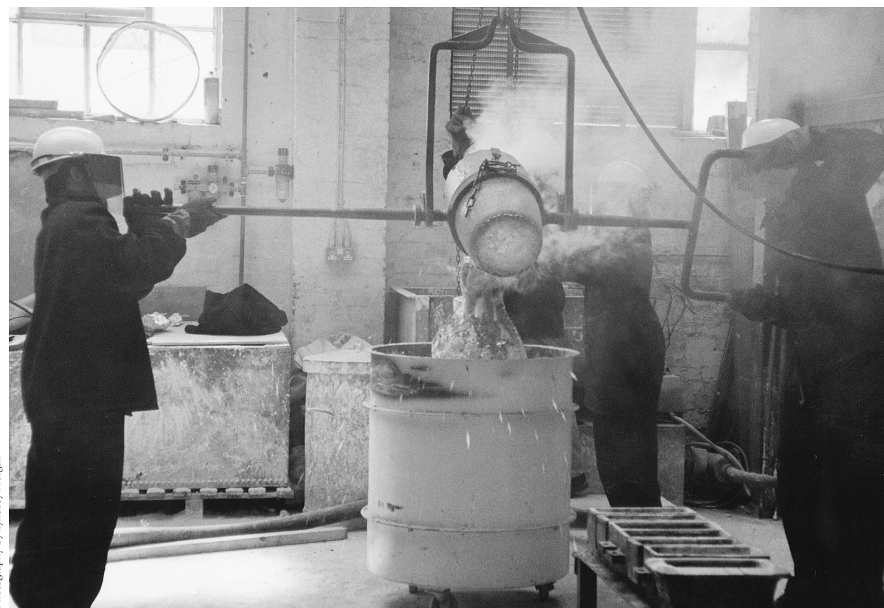
Figure 1. Bronze samples being cast in the foundry of the RCA Sculpture School.
