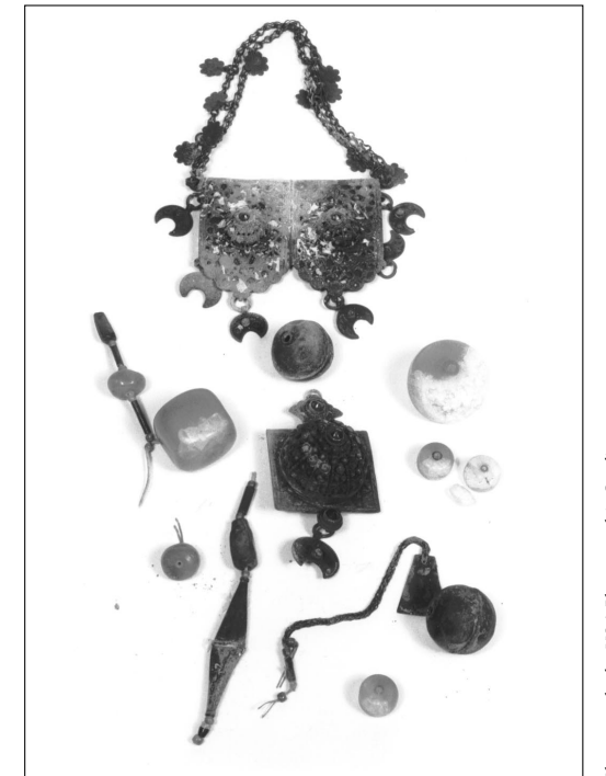
Figure 4. Badly degraded cellulose nitrate and metal necklace from 1922 stage production of Chu Chin Chow .
