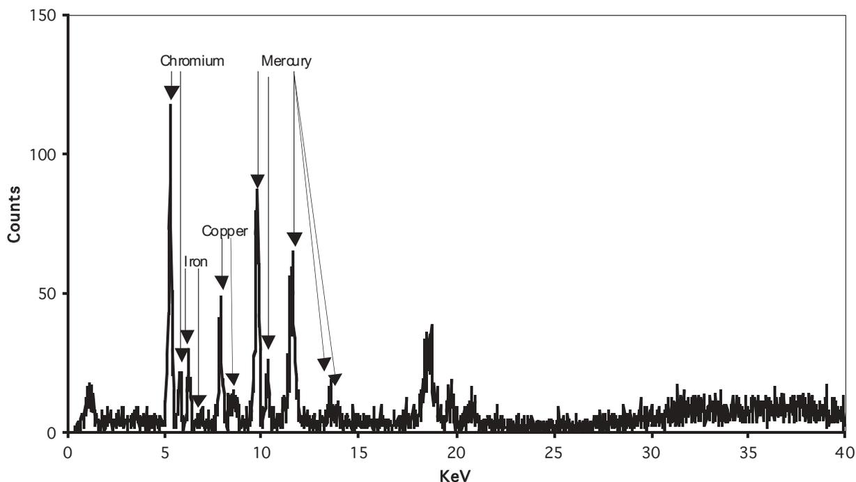
Figure 2. EDXRF spectrum of T.105-1937 showing mercury and also note chromium content.
