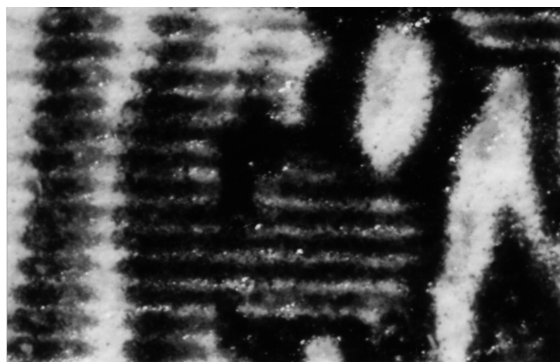
Figure 3. The striated surface of the image layer on a colour photocopy. Colours are created by layering differently coloured "glazes" of pigment bound in toner on top of each other. (magnification x60 approx.)
