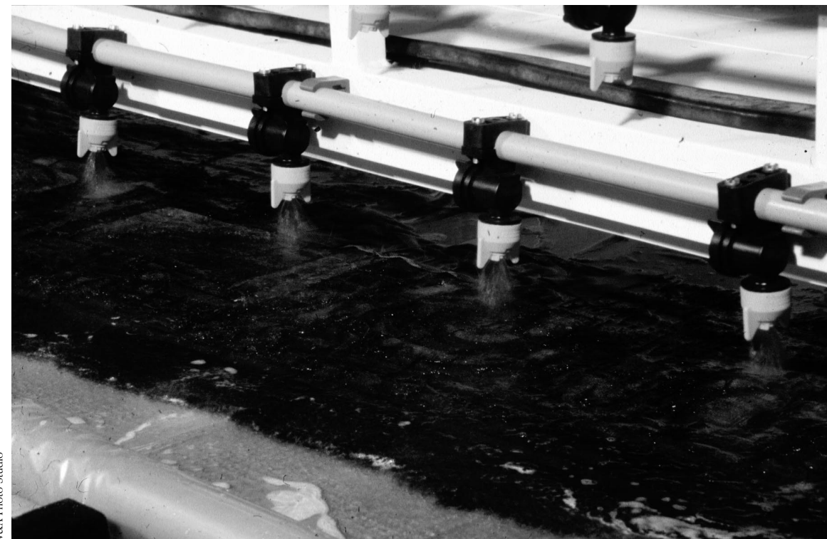
Figure 3. Detail of the nozzles on the spray bar
