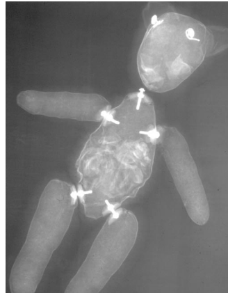
Fig 2b X-radiograph of teddy showing position of attachment bolt for head
