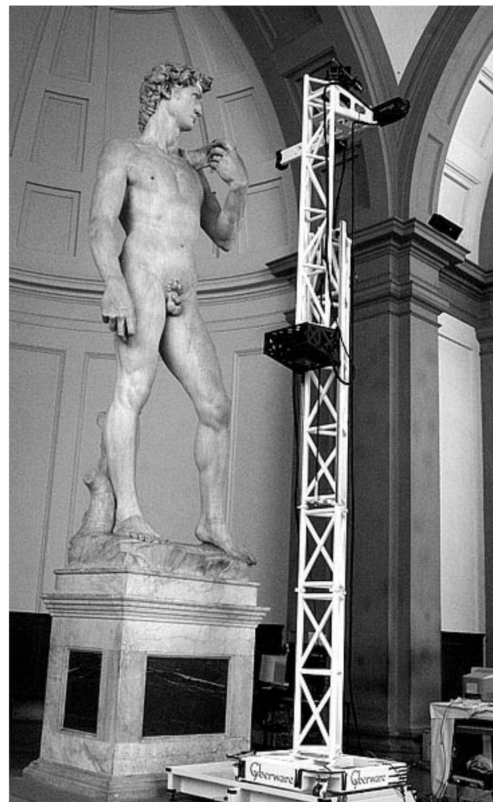
Figure 3: The scanner from Cyberware® scanning "David" reproduced courtesy of the Digital Michelangelo Project, Stanford University
