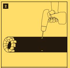
File down and pad the ends with foam and gaffer tape, and drill holes in both sides.
