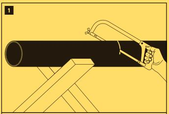
Use a hacksaw to cut the metal pipe into lengths of about 4 ft. shorter ones are possible, but make access to the 'cuffs' easier.
