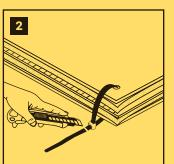
Secure the side holes tightly with cable ties. Cut off the ends that are sticking out.
