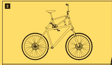
Sit one bike on top of the other and weld them together. Add extra material to strengthen, and join the forks together so the top bike steers the bottom. Add a new chain and brakes so the top bike drives the bottom one. Repeat with two more bikes. The pair of top bikes and the pair of bottom bikes should match as closely as possible.
