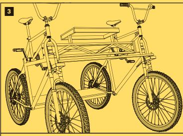
Weld in a connecting frame for people to stand on, and another near the front of the bike to make the entire unit into a rigid structure.
