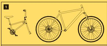
Remove wheels, chain and brakes from the top bike. Cut off the seat stay and chain. Remove handlebars and seat post from bottom bike.
