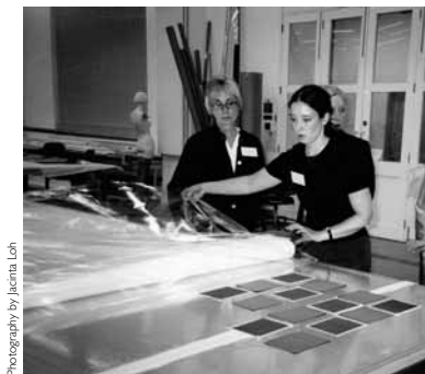
Figure 1. Using the vacuum hot table for application of adhesive
