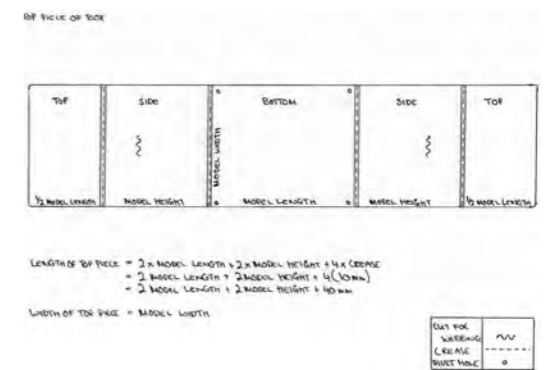
Figure 2. Template for the top piece of the box
