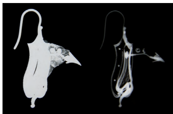
Figure 3. An X-ray showing the internal structure of the earring at 35KV and the metal wires at a higher KV
