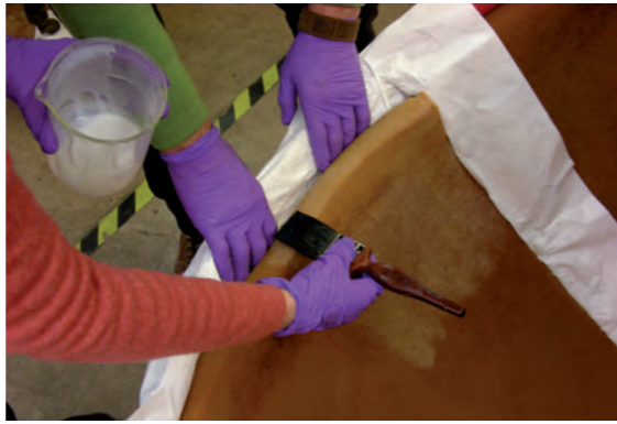
Figure 2. Applying Impranal® DLV to the chair
